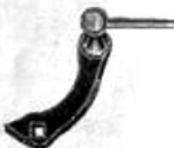
"PHILLIPS" BRAKE ROD, with lug and lever stop, for Rear roller brakes.
