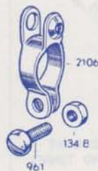
(Code No. 1091), Ref. 2112. CABLE (O/Casing) STOP, fits on Rear Chainstay.
