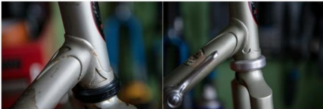
Prugnat S4 and 62D Head Lugs My TI-Raleigh SBDU Ilkeston
