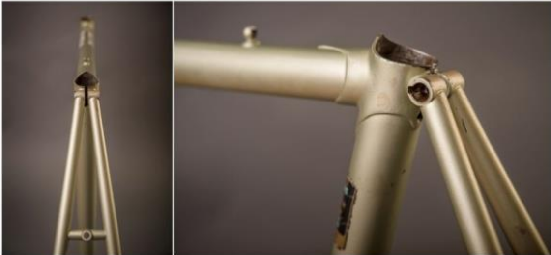
Raleigh SBDU Ilkeston Time Trial Special 1982 SB5464 Shot in Stays
