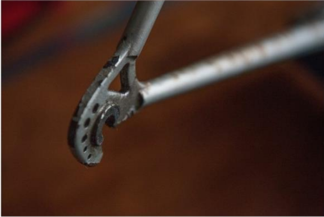
Campagnolo 1060 Vertical Drilled Rear End My TI-Raleigh SBDU Ilkeston
