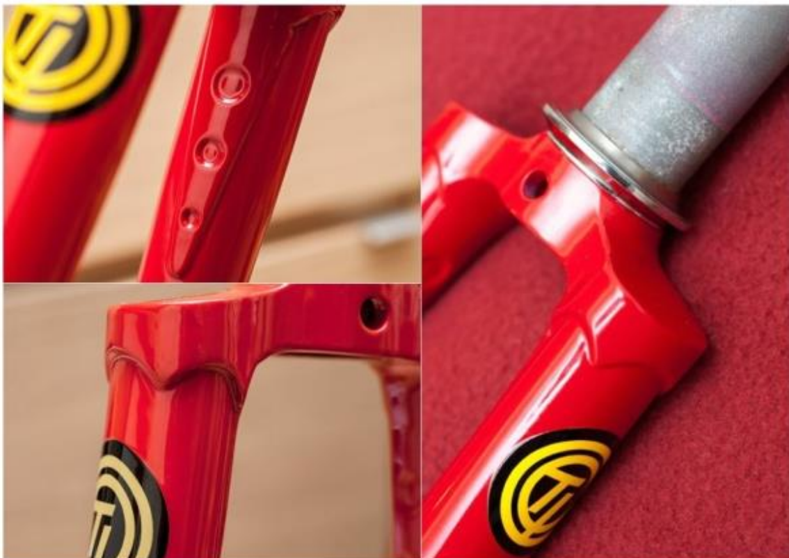
Fork Crown with Stiffener Tang My TI-Raleigh SBDU Ilkeston
