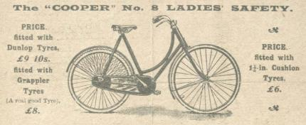
SPRCIFICATION .- Large Diameter Weldless Steel Tubes throughout ; Wheels, driver 26in., front 2Sin. ; Chun. Best. Block; Spokes, Tangent, High Tension, Plated; Penals, Rubber; Detachable Rubber Brake; Geared 55in, to bin, or to order; Weight, about 34bs.; fitted w Transparent Gear Case; Wheel and Dress Guards; Enamelled Black, with usual parts Plated in Best J.e.
