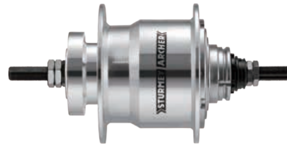
X-RK4 4-Speed · Disc Brake Hub
