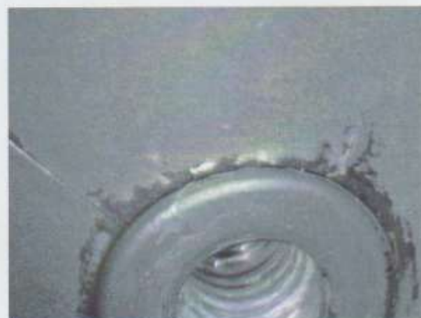
Figure 5: Example of Over-Torqued Rivet Nut that Lead to Frame Failure
