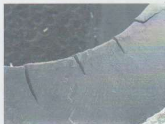
Figure 6: SEM Photograph Showing Mechanical Deformation Caused by Over-Torqued Rivet Nut
