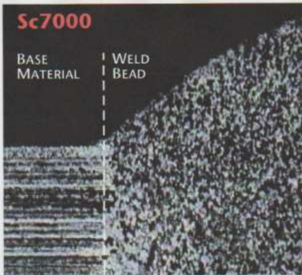
Figure 1: SC7000 Base Material and Scandium Weld Rod
