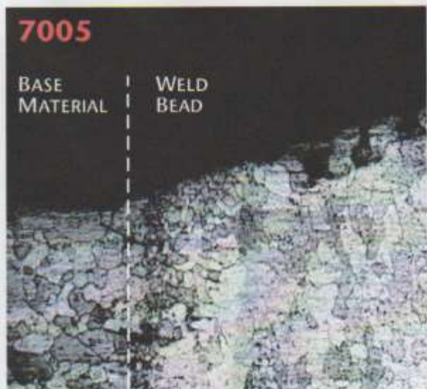
Figure 2: 7005 Base Material and 5356 Filler Rod
