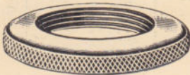
BSR 598 Screwed ball race \frac{31}{32} " x 30 threads, for \frac{1}{8} " balls. BSR 632 ditto, for 1" x 24 threads. BSR 601 ditto, for 1" x 26 threads. BSR 107 ditto, for \frac{1}{8} " balls and 1" x 24 threads.
