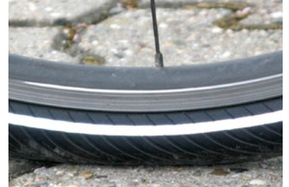
That’s how it should look. The tire is hardly deformed under the weight of the rider.
