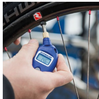
Inflation pressure check with the Airmax Pro.
