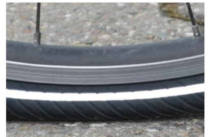
That’s how it shouldn’t look. The inflation pressure is far too low here.
