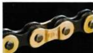
The UG Chain. Outer plates are widened to the level of chainpin heads.
