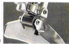
Trapezium shaped swing motion of Trap-Ease Mechanism
