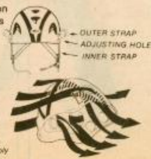
Arrows show air-cooling flow through helmet.
