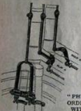
FRONT AND REAR BRAKES Fitted with Roller Levers on Handlebar. Clip (A) Fitting Bell Crank.
