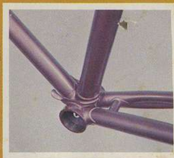
Investment cast BB shell, cut-out with Colnago clover logo, Campy cable guides, massive Columbus chain stay, both models with wheel indentation.
