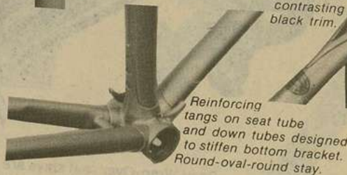
Distinctive Haden lugs are extra-thin with perfect edges.
