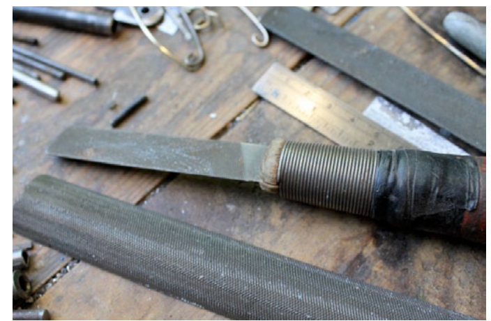
Some files are shortened to make them more suitable for certain tasks
