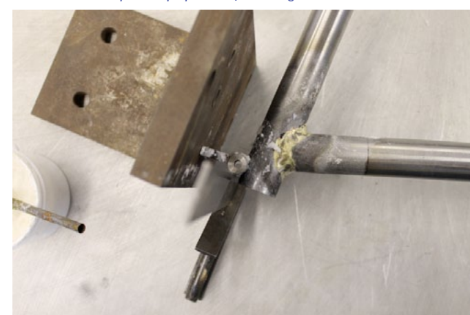
Ensuring that the seat binder is square to the alignment table.
