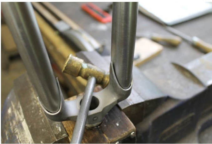
Using a brass hammer to improve the fit between the fork crown and blades.
