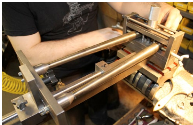
Unicrown fork jig. The fork blades are held at the bottom on cones, before the dropouts are added.
