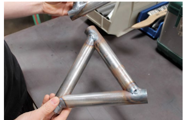
This triangular practice piece is used for Tig welding.
