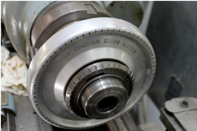
Another lathe with a rubber-flex collet.
