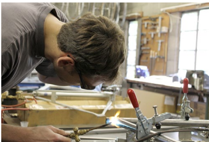
Taking the main tubes in place with brass.
