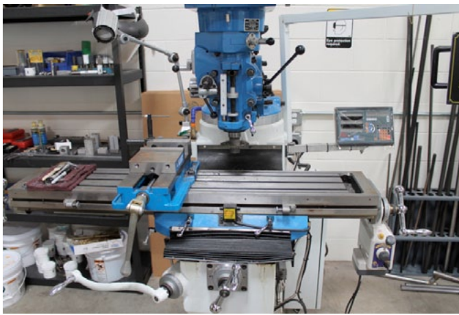
Main tube mitring is done on this milling machine.
