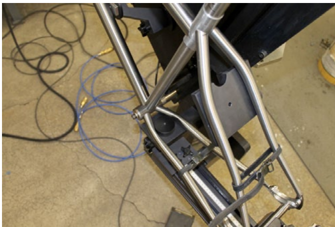
Carefully bent stays.
