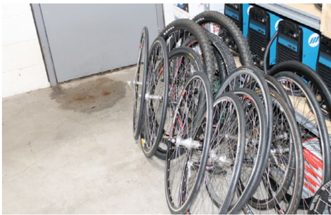
Trued and perfectly dished wheels for checking alignment when building frame rear triangles.
