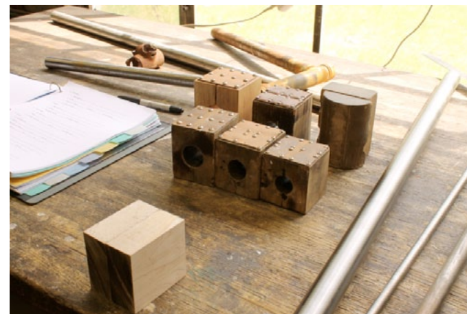
Tubing blocks for different sized tubes, made of hard maple.
