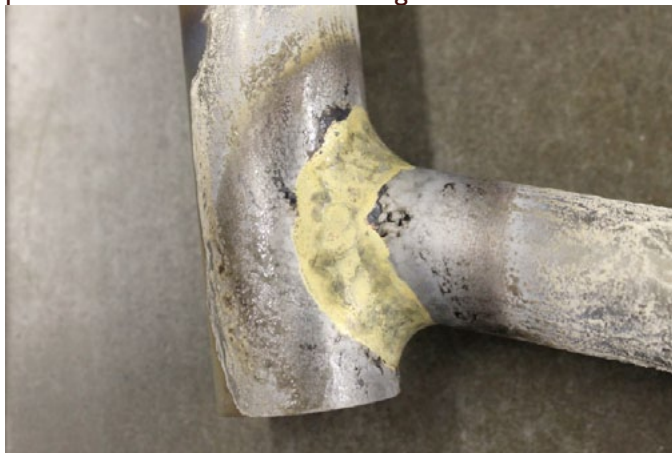
A freshly fillet-brazed joint – still caked in protective flux.
