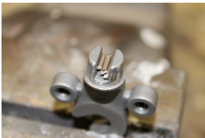
Loading the plug-in dropouts with bits of silver.
