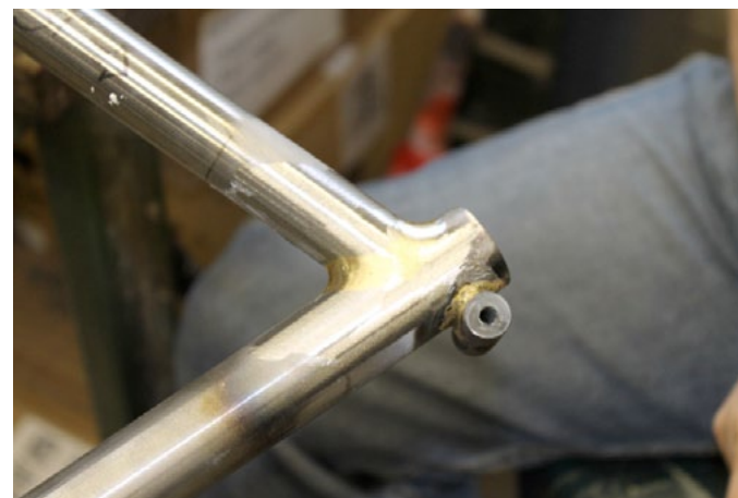
The fillets look nice after a buzz with the Dynafile.
