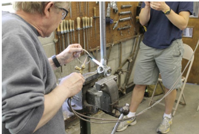
Doug cleans the 'shoreline' of the bottom bracket shell with the flame.
