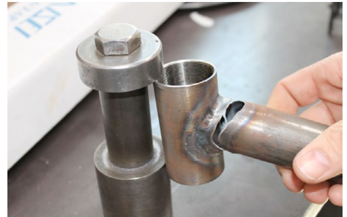
The welded or brazed joins are then tested by inserting a bar and levered on. A break on the weld = failure. Above the weld = good join.
