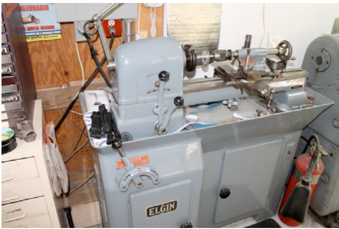
A lathe with constantly variable speed.
