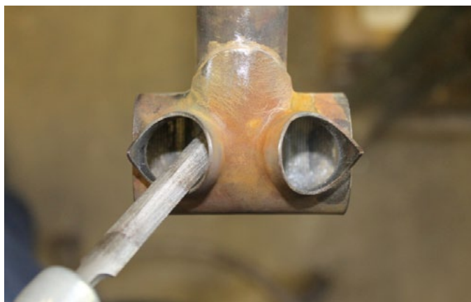
Filing the chainstay sockets: The surface rust is only a very thin layer - caused by soaking off the flux in hot water after brazing. It's honest American rust.
