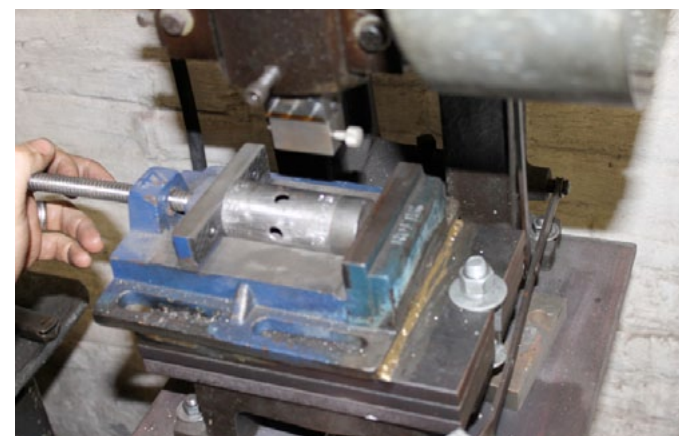
The press in action on a bottom bracket shell. Bearing cups or machined substitutes are inserted into the press to prevent distortion of the shell.
