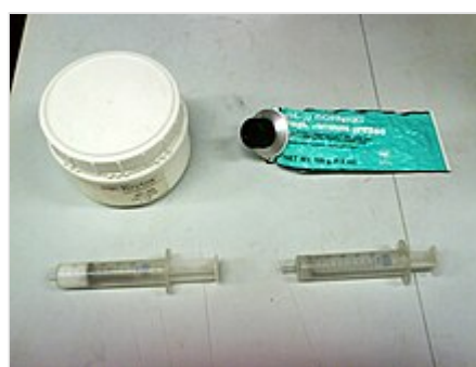
Grease is used to lubricate glass stopcocks and joints. Some laboratories fill them into syringes for easy application. Two typical examples: Left - Krytox , a fluoroether-based grease; Right - a silicone-based high vacuum grease by Dow Corning .
