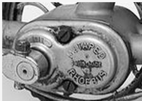
The 1937 bracket used 2 bolts.
