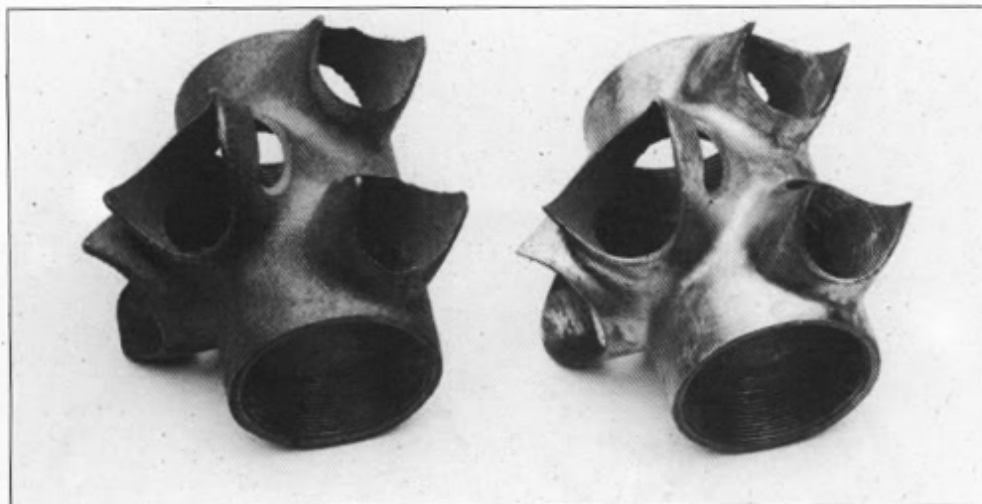
FISCHER BOTTOM BRACKET SHELL (MASI STYLE, FROM 1973) READY FOR FILING
