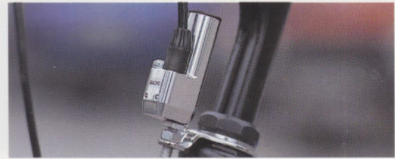
Retrofit hydraulic power boost with the Sachs Hydraulic Power Cable.
