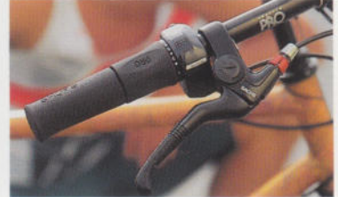
Power Grip Pro: two-part twist grip.
