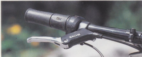
Sachs' completely new hydraulic brake lever is available in 2- and 4-finger versions (2-finger version above here).
