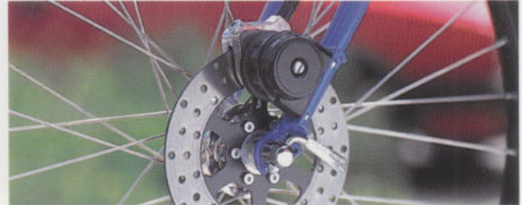
Hydraulic Disc Brake: the braking system of choice for state-of-the-art mountain bikes.
