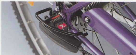
The Click Box simplifies wheel changes and eliminates re-adjusting.
