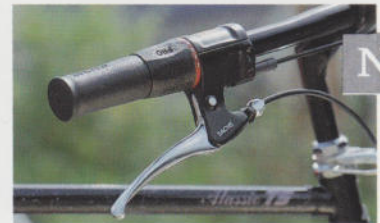
Power Grip Pro for Pentasport and Super 7 (Super 7 above here).
