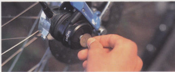
Brake pads are easy to adjust.
