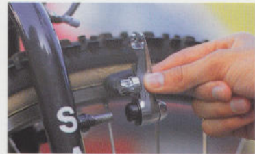
Pre-assembled spring unit make it easy to install and adjust cantilevers.
