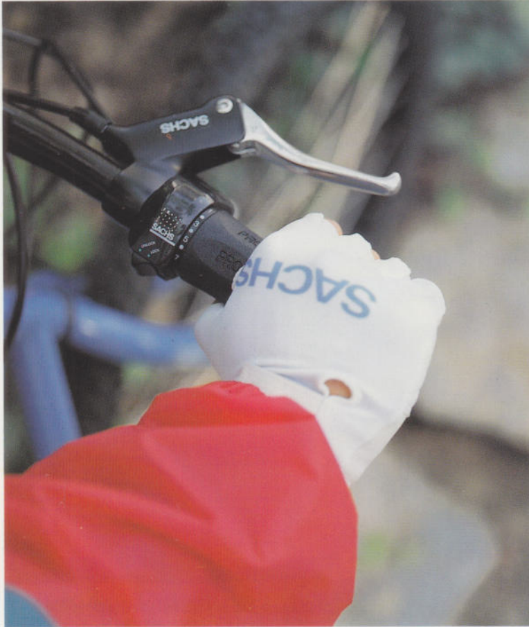
Power Grip Pro: two-part twist grip.
