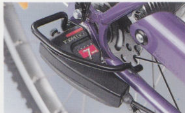
Click-Box: Factory adjusted for perfekt shifting
