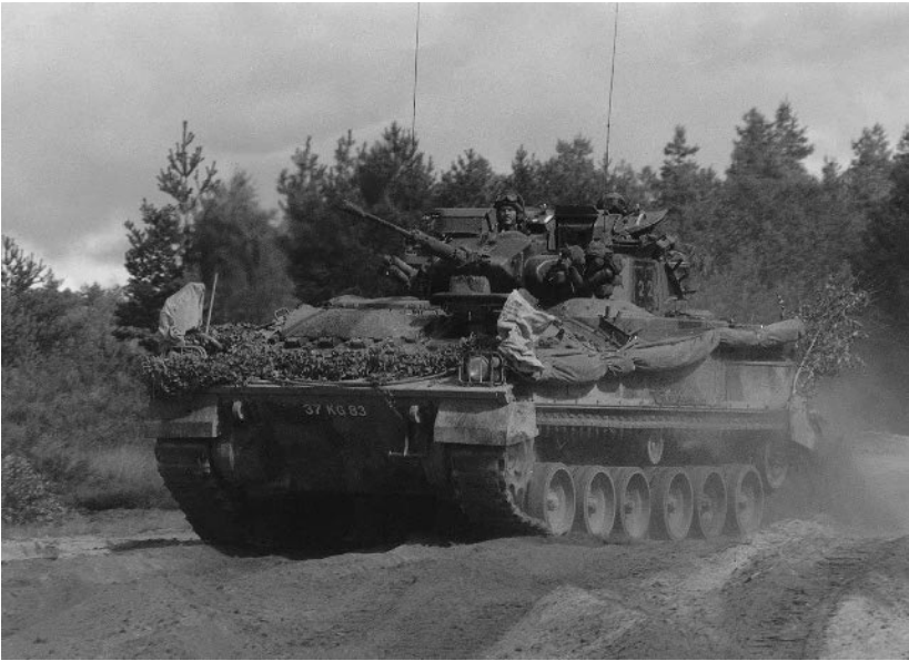
1.3 Warrior armoured fighting vehicle (AFV) utilising Al-Zn-Mg alloys. Courtesy of Alvis Vehicles.
