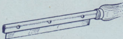
The simply made holder for use with broken hacksaw blades
