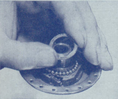
Slipping on a shim for free wheel adjustment
