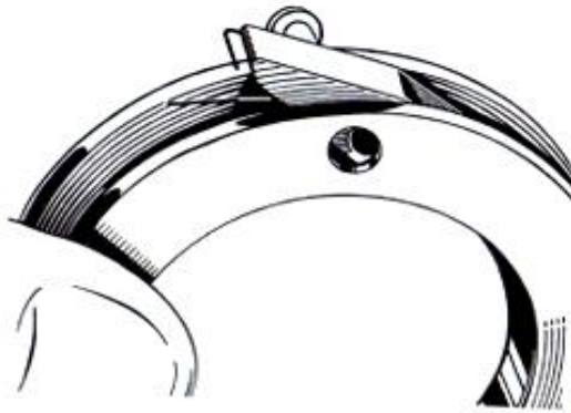
Fitting pawl and spring to planet cage pawl ring—TCW.
