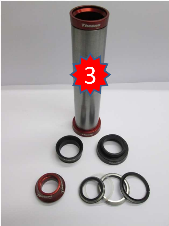
HEAD SET FIXED BY PRESS TOP "ø48 x 15 + 10" mm BOTTOM "ø58 x 12" mm
