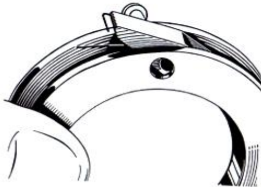
Fitting pawl and spring to planet cage pawl ring—TCW.
