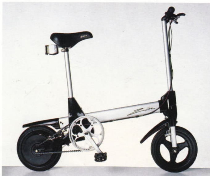
Where's the battery? In the front cross member.
