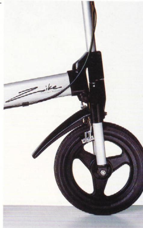
The frame construction is aluminium alloy and 'Verton' from ICI Materials.
