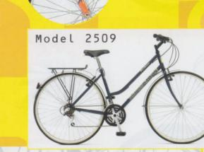
Model 2508 / 2509 Hi tensile steel lightweight Town & Trail frame design Shimano 18 speed gears with gripshift controls 'V' style brakes and alloy silver rims Fitted with mudguards and rear carrier 21" 23" 2509 Frame size 18" 20" 2508 Frame size
